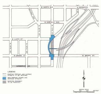
ALTERNATIVE NO. 8 FOR COMPLETION OF THE HILLSIDE INTERCHANGE NORTHERN SPUR
