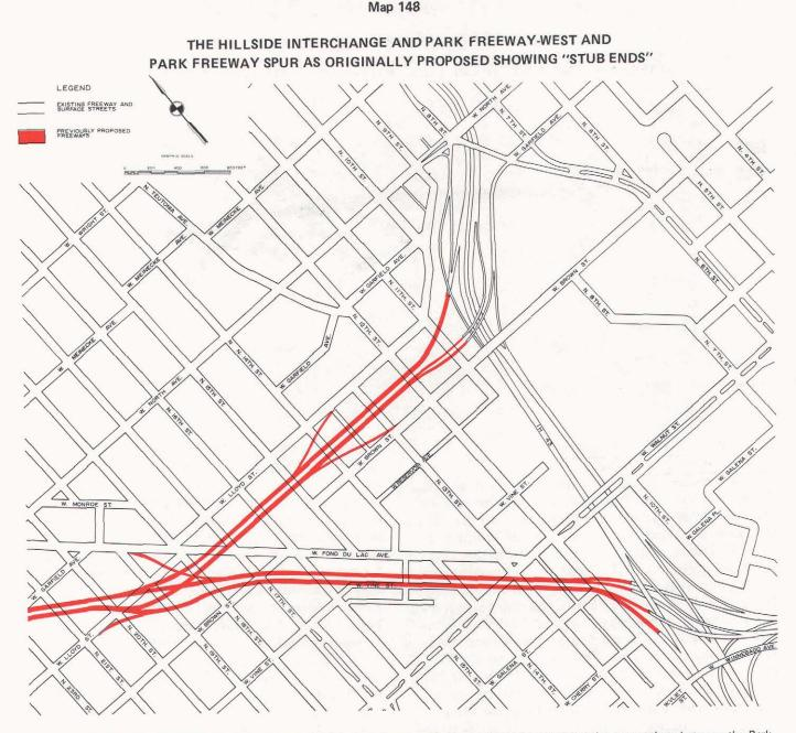
As shown on this map, as originally proposed, the Hillside Interchange and spur was to have provided the connections between the Park Freeways-East and West and the North-South Freeway (IH 43). As a result of the removal of the Park Freeway-West and Park Freeway spur from the regional and, subsequently, the state and local transportation system plans, the Hillside Interchange and spur were left with seven "stub ends."
