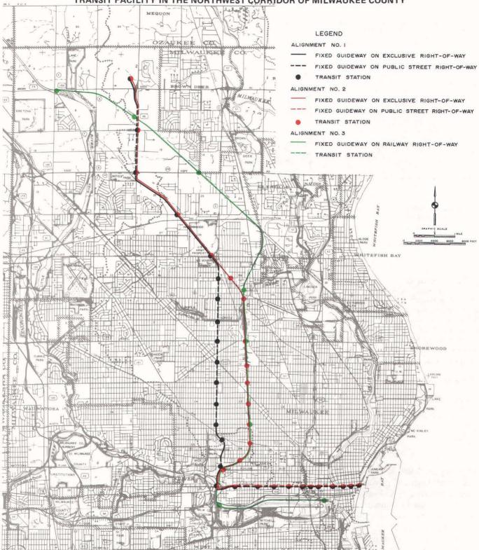
THREE ALTERNATIVE ALIGNMENTS FOR THE RECOMMENDED LIGHT RAIL TRANSIT FACILITY IN THE NORTHWEST CORRIDOR OF MILWAUKEE COUNTY
