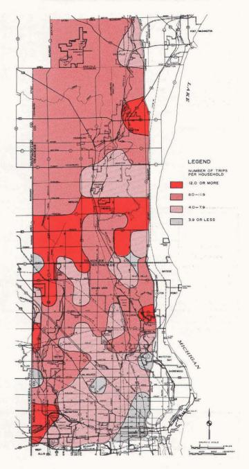
This map shows the variation within the study area in household trip generation on an average weekday in 1972. A low tripmaking rate is evident in the central area of the City of Milwaukee and in a few scattered rural areas, and higher than average tripmaking rates are evident in the suburban and rural-urban fringe areas of the study area. Differences in automobile availability, household size, and household income between these areas explain these differences in tripmaking.
