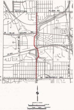
This map shows the proposed alignment of a new roadway which would be situated along N. 124th Street extended between W. Greenfield Avenue and W. Watertown Plank Road. Completion of this segment of N. 124th Street would help to abate traffic congestion in the north-south travel corridor in the western portion of the study area.
