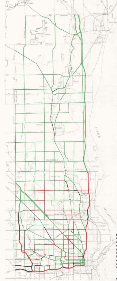
VOLUME-TO-CAPACITY RATIOS ON THE ARTERIAL STREET AND HIGHWAY SYSTEM IN THE NORTHWEST SIDE STUDY AREA DURING THE EVENING PEAK HOUR: 1978
