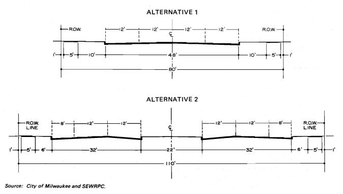
TYPICAL CROSS-SECTIONS OF IMPROVEMENT ALTERNATIVES 1 AND 2 FOR N. 91ST STREET FROM W. MILL ROAD TO W. BRADLEY ROAD
