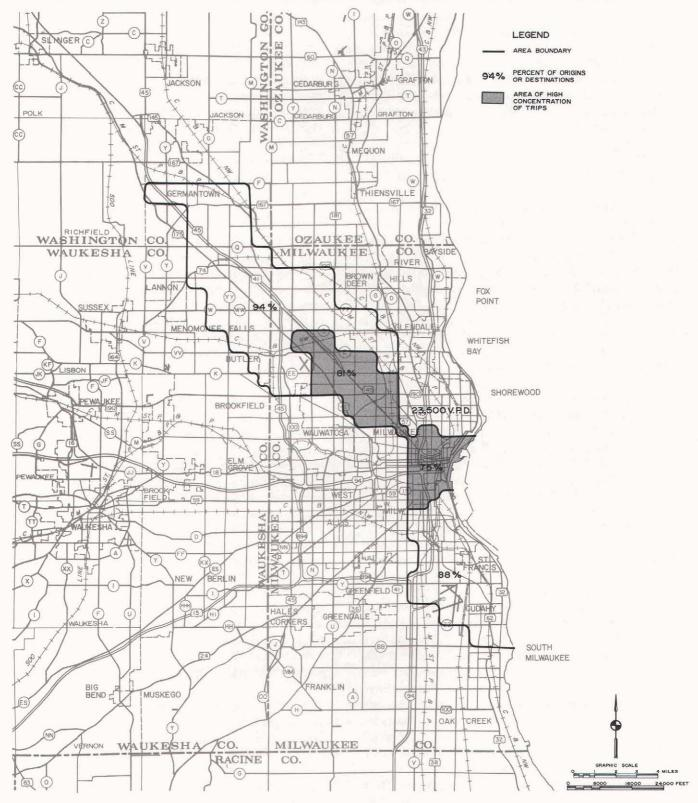
PROJECTED TRIP ORIGINS AND DESTINATIONS OF VEHICLES TRAVERSING THE SEGMENT OF W. FOND DU LAC AVENUE BETWEEN N. 27TH STREET AND N. 21ST STREET UNDER THE RECOMMENDED ALTERNATIVE
