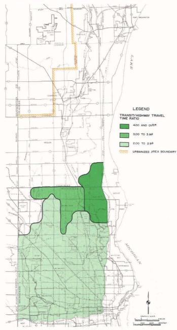
Ideally, overall travel time on the public transit system should be similar to overall travel time by automobile between component parts of the study area and between component parts of the area and the remainder of the Milwaukee transit service area. As shown on this map, the average midday travel time on public transit from those parts of the northwest side study area served by public transit would generally be two to three times greater than travel time for equivalent trips by automobile.
