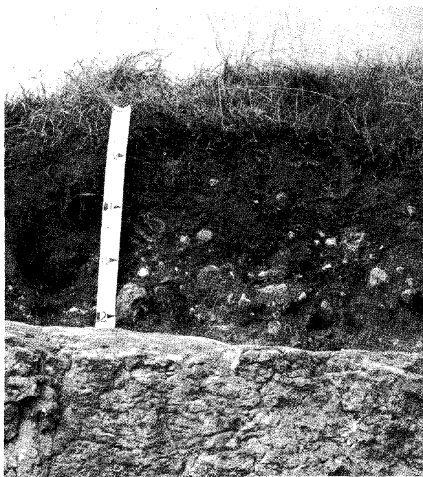
The silty Knowles soils are underlain by dolomite bedrock at less than 3 feet. The soil material has low bearing capacity, moderate to high shrink-swell capacity, a low percolation rate and a moderate frost hazard.
