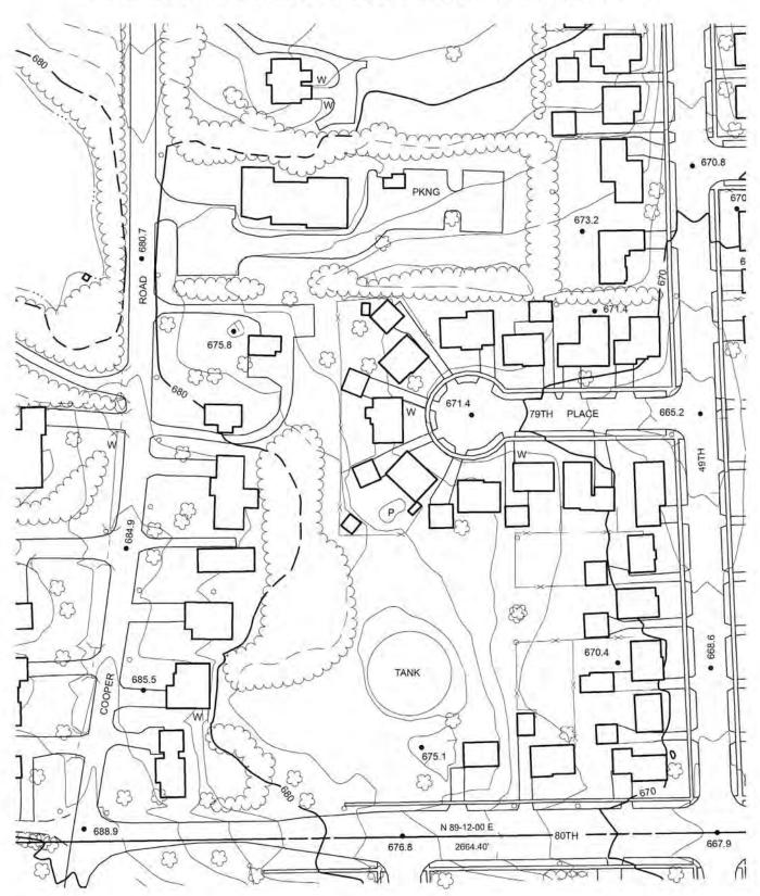
PORTION OF TYPICAL LARGE-SCALE TOPOGRAPHIC MAP AT ONE INCH EQUALS 100 FEET
