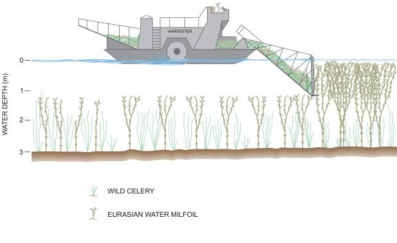
PLANT CANOPY REMOVAL WITH AN AQUATIC PLANT HARVESTER
