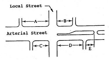
Minimum Desirable Corner Clearances at an Arterial and Local Street Intersection Controlled by Stop Signs on the Local Street
