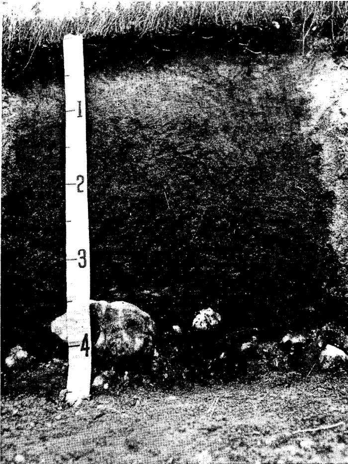
Figure 7.—Profile of a Dodge silt loam. This soil formed in silt and loamy glacial till.
