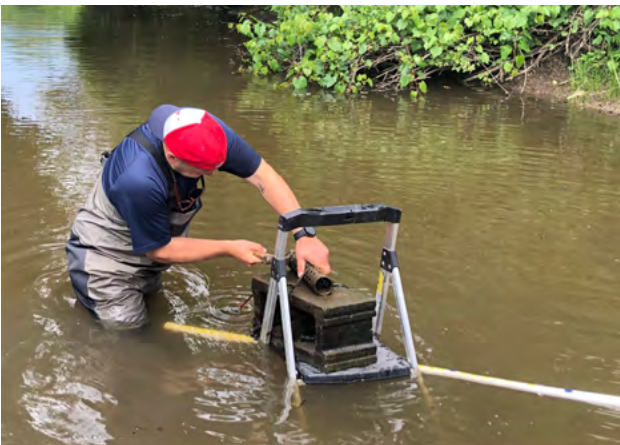
The stream sensors required periodic cleaning for sediment, debris, and small aquatic organisms
