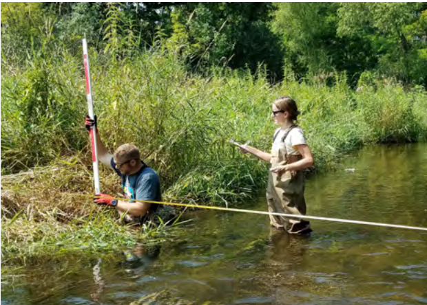
Commission staff collecting data for streamflow measurements at a sampling location
