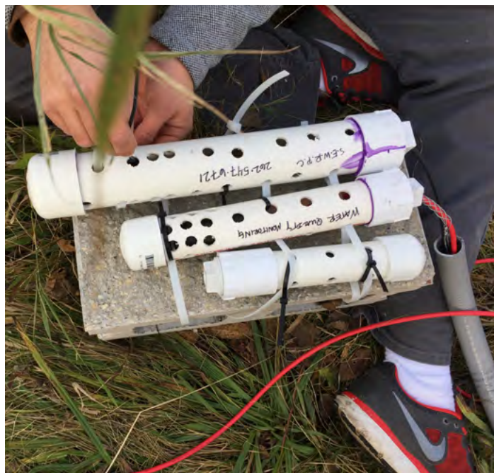
PEWAUKEE RIVER PILOT MONITORING SITE – SENSOR CONFIGURATION
