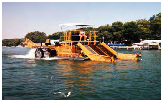
Figure 2.75 Lake Pewaukee Sanitary District Aquatic Plant Harvester
