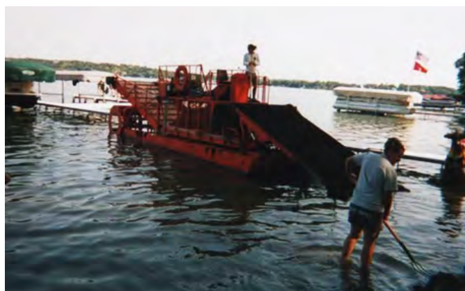
Figure 2.77 Lake Pewaukee Sanitary District Small-Scale Aquatic Plant Harvester
