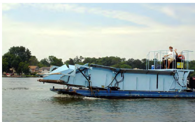
Figure 2.76 Lake Pewaukee Sanitary District Aquatic Plant Transport Barge
