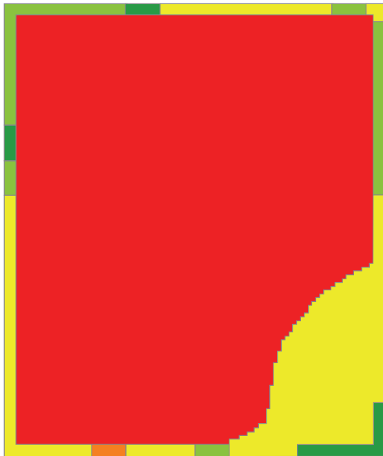
Figure 11. Distribution of horizontal hydraulic conductivity in child model, layers 1 and 2.
