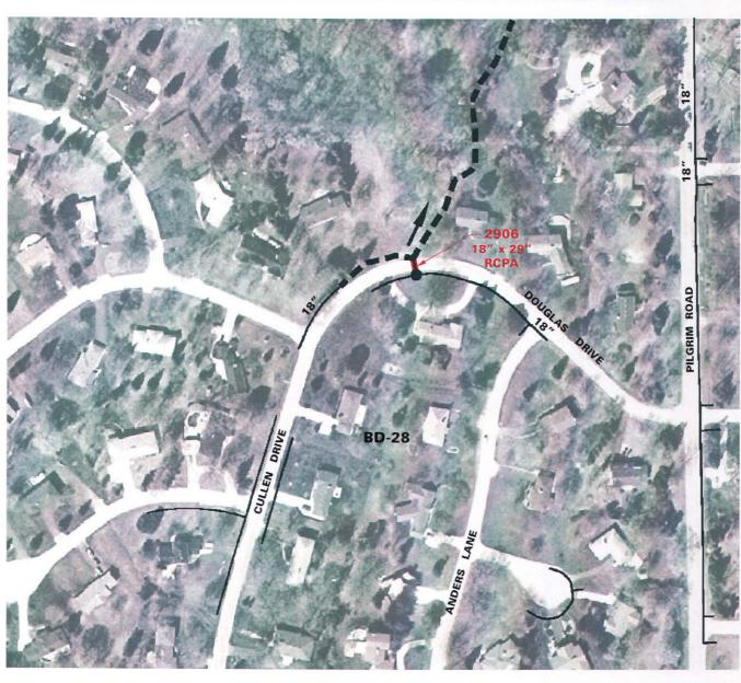
REINFORCED CONCRETE PIPE ARCH
