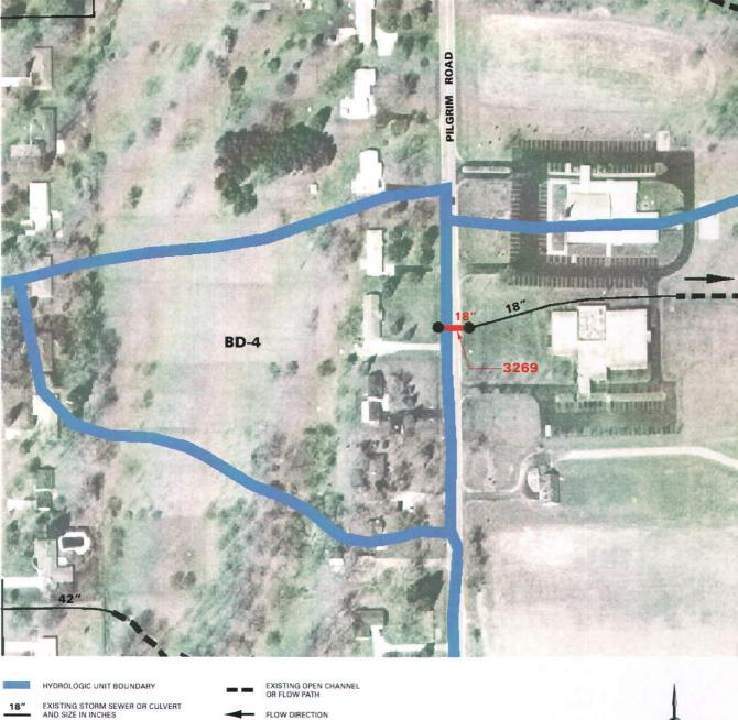
THIS MAP GENERALLY SHOWS STORM SEWERS OF 18 - INCH DIAMETER OR LARGER. PIPES ARE REINFORCED CONCRETE UNLESS STATED OTHERWISE
