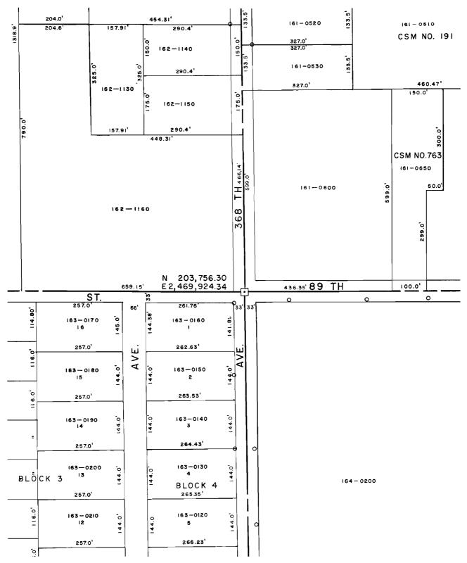
Shown here at drafted scale (1 inch equals 200 feet) is a portion of the cadastral map prepared for Section 16 in the Town of Randall, Kenosha County. The figure is roughly centered on the center of the section and encompasses an area of approximately 50 acres, or about 8 percent of the area covered by the full map. A topographic map of the same area is shown in Figure 6.
