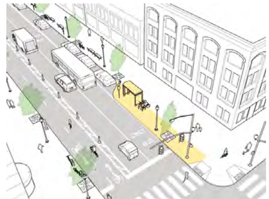
Illustration of a Bus Bulb (in Yellow)
