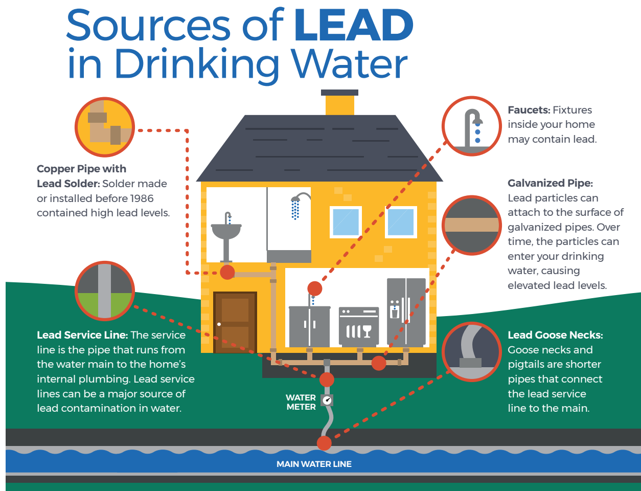
Figure 3 Potential Sources of Lead in Household Plumbing
