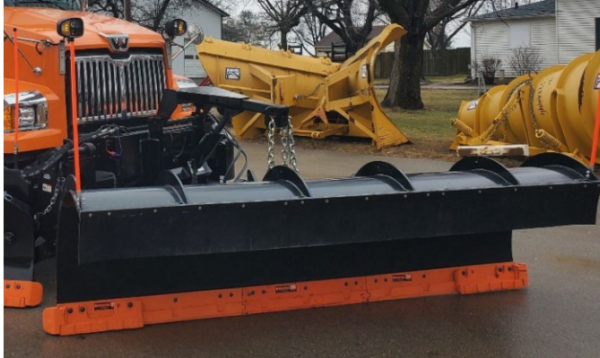
Sectional Blades on a Front-Mounted Plow
