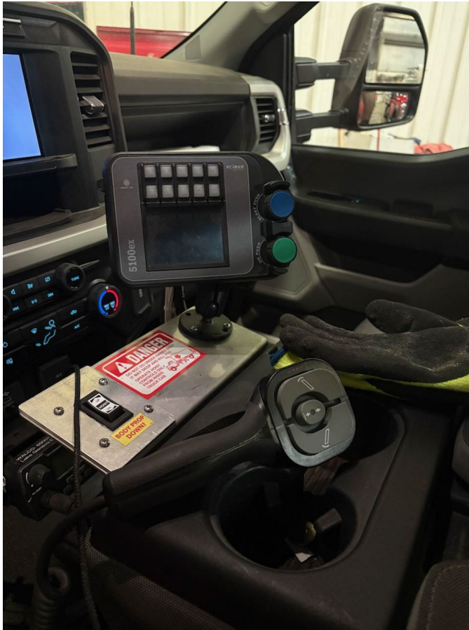
Figure 8.8 In-Cab Electronic Controller System
