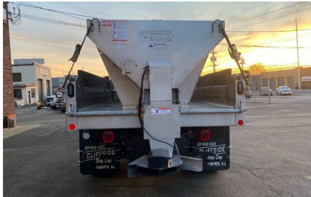
Directional Spinner Mounted on V-Box Spreader
