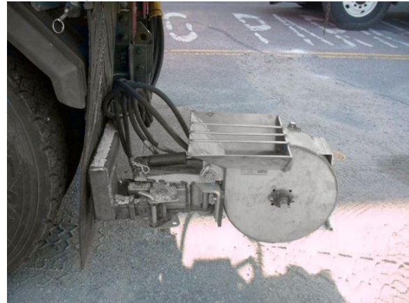
Zero Velocity Spreader
