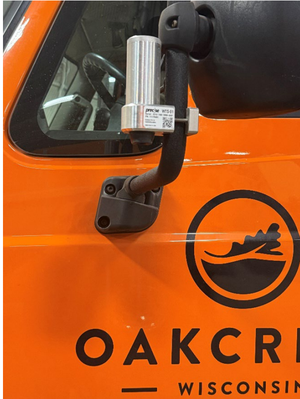
Figure 8.2 Truck-Mounted Mobile Infrared Pavement Temperature Sensor and In-Cab Display
