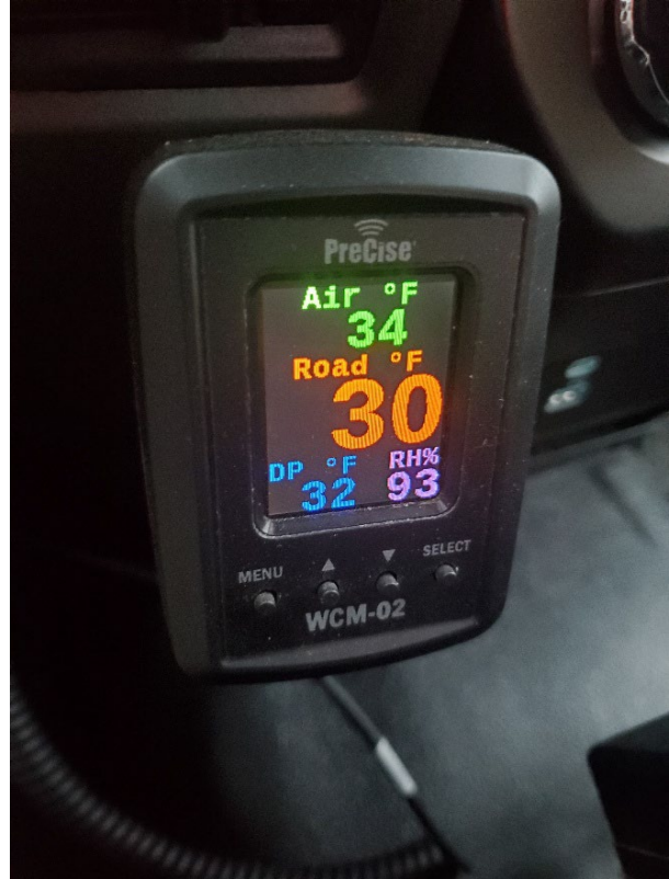
Figure 8.2 Truck-Mounted Mobile Infrared Pavement Temperature Sensor and In-Cab Display
