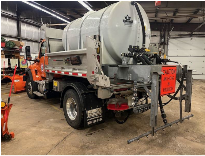
Figure 8.6 Anti-Icing and Direct Liquid Application Rigs and Tankers
