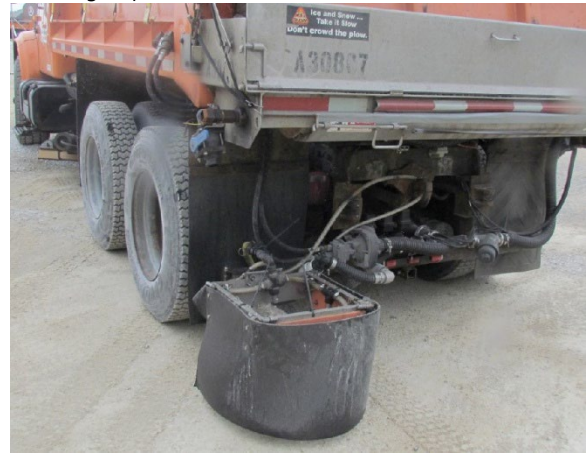
Zero Velocity Spreader
