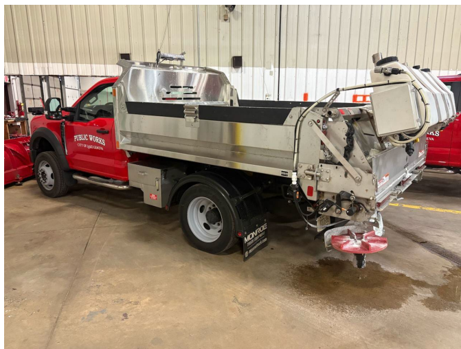
Figure 8.5 Examples of Pre-Wetted Salt Spreaders
