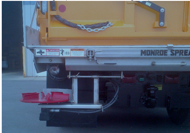
Directional Spinner Mounted on V-Box Spreader
