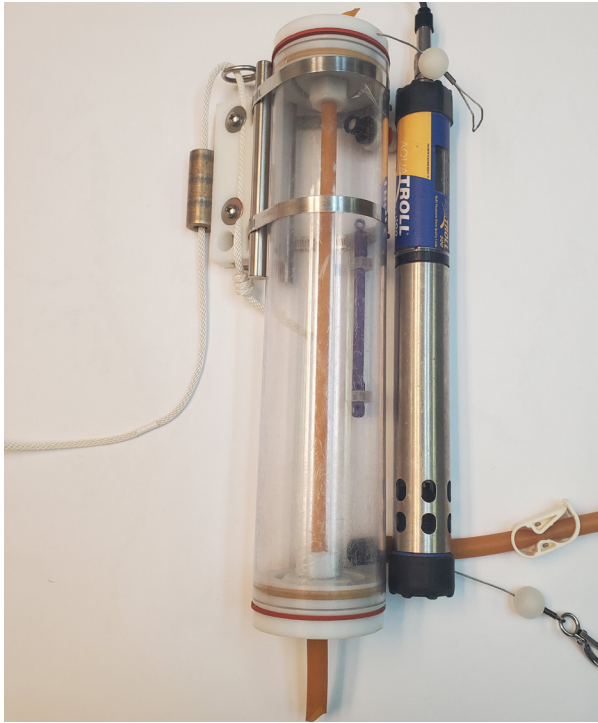
Figure 7.3 Niskin-Style Vertical Water Sampler and Aqua TROLL 500 Multiparameter Sonde Assembly
