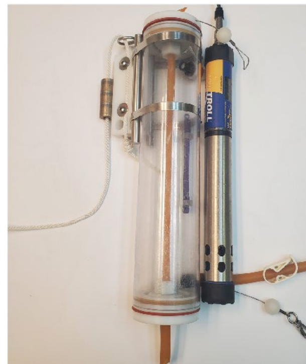
Figure 7.3 Niskin-Style Vertical Water Sampler and Aqua TROLL 500 Multiparameter Sonde Assembly
