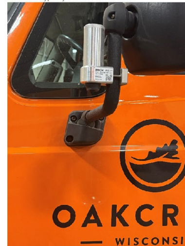
Figure 2.11 Truck-Mounted Mobile Infrared Pavement Temperature Sensor and In-Cab Display
