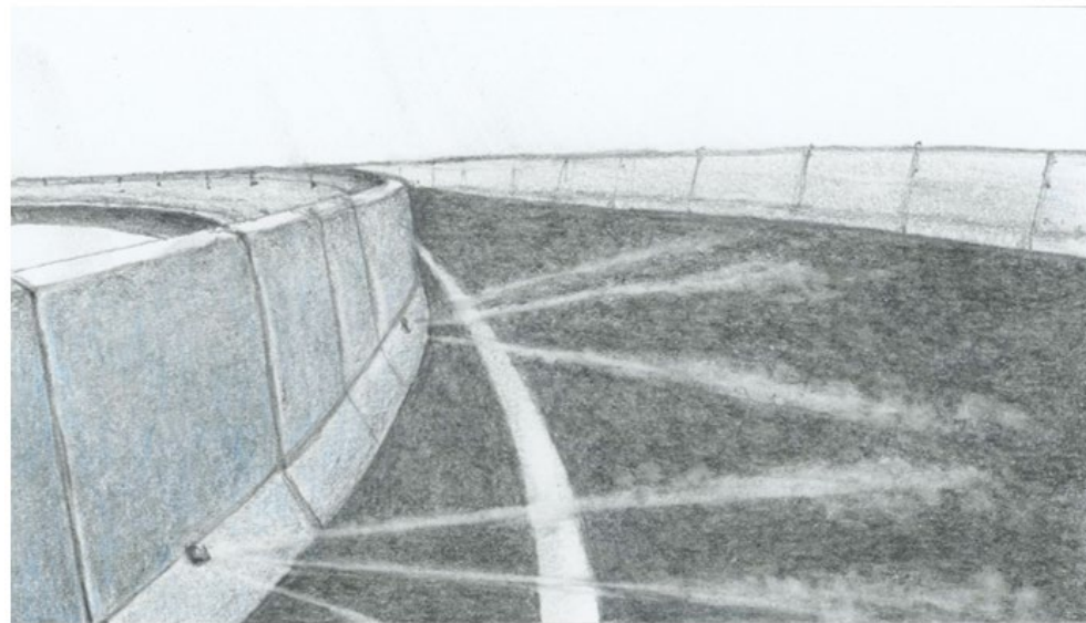
Figure 2.31 Fixed Automated Spray Technology (FAST) System for Brine Application
