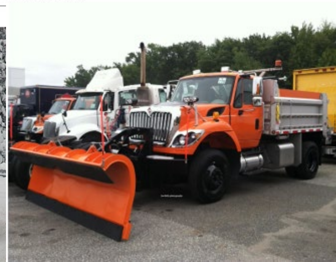
Figure-2.131 Front-Mounted-Reversible-Plow with-Wing-Plow-Attachment
