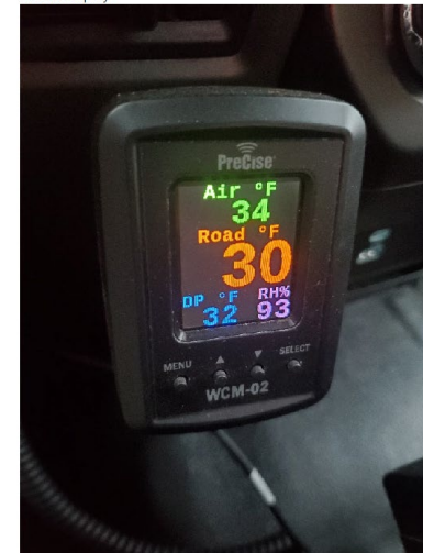
Figure 2.11 Truck-Mounted Mobile Infrared Pavement Temperature Sensor and In-Cab Display
