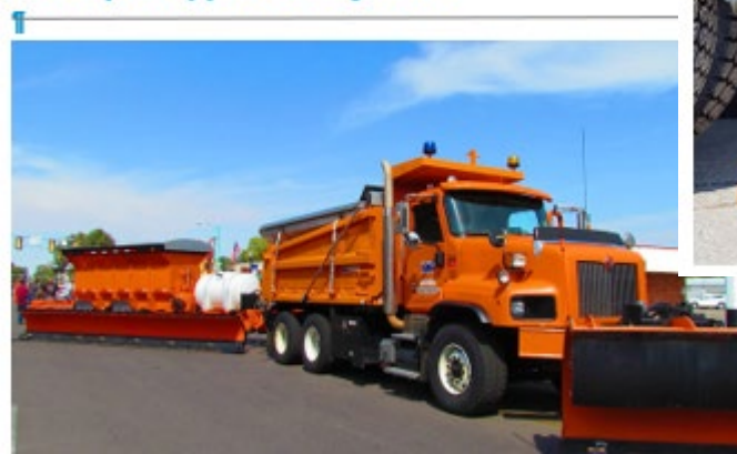
Figure-2.151 Example-a-Tow-Plow-Attachment-with-Solid and-Liquid-Application-System
