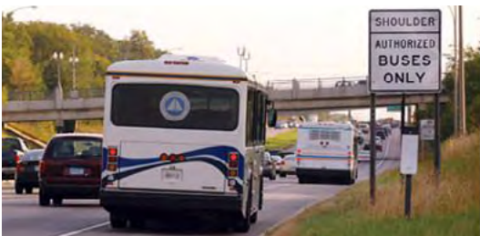
Bus-on-shoulder Credit: Minnesota Department of Transportation
