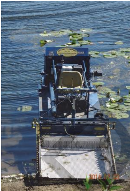
Hockey Underwater Cutter (photo: SEWRPC 2014)
