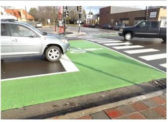
An intersection in Wauwatosa, Wisconsin utilizing a bike box at the head of a traffic lane
