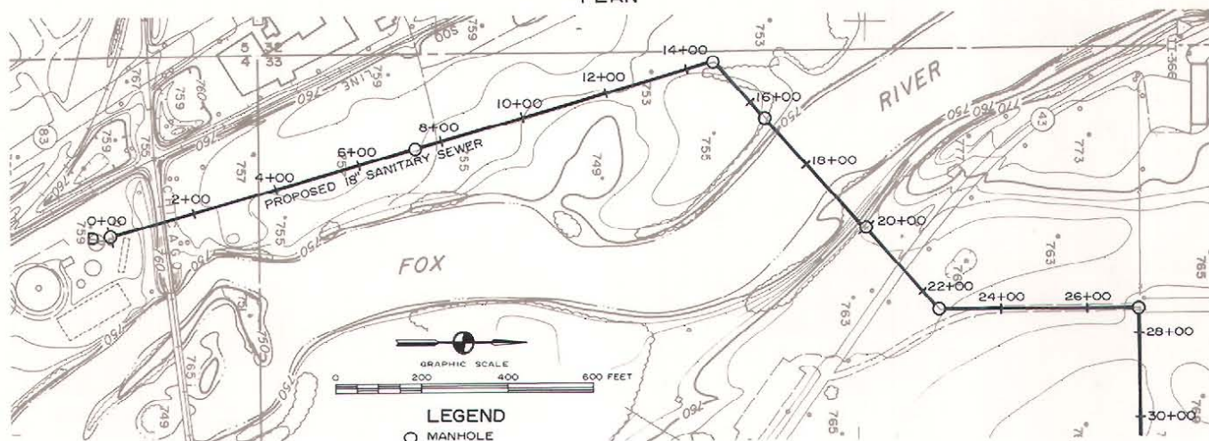
Figure 23 (continued) RECOMMENDED SANITARY SEWERAGE FACILITIES FOR BROWNS LAKE: ENTIRE LAKE WITH TREATMENT PLANT AT BURLINGTON
