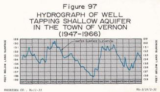
William M. Foss. NW4 Section 2, T.5N., R.19E. Drilled unused artesian well in the Niagara dolomite aquifer, diameter 6 inches, depth 508 ft., cased to 434, elevation of land surface 962 ft. above msl. top of casing, 1.00 ft. above land surface. Recording age. Lowest monthly elevation plotted.
