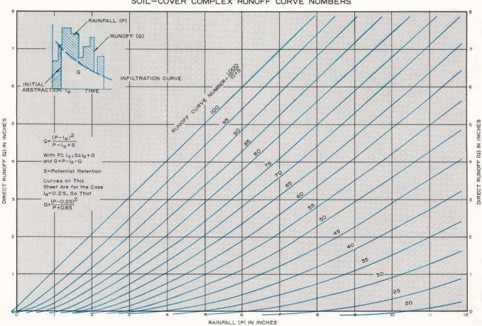
Figure 44 RAINFALL-RUNOFF RELATIONSHIPS FOR HYDROLOGIC SOIL-COVER COMPLEX RUNOFF CURVE NUMBERS
