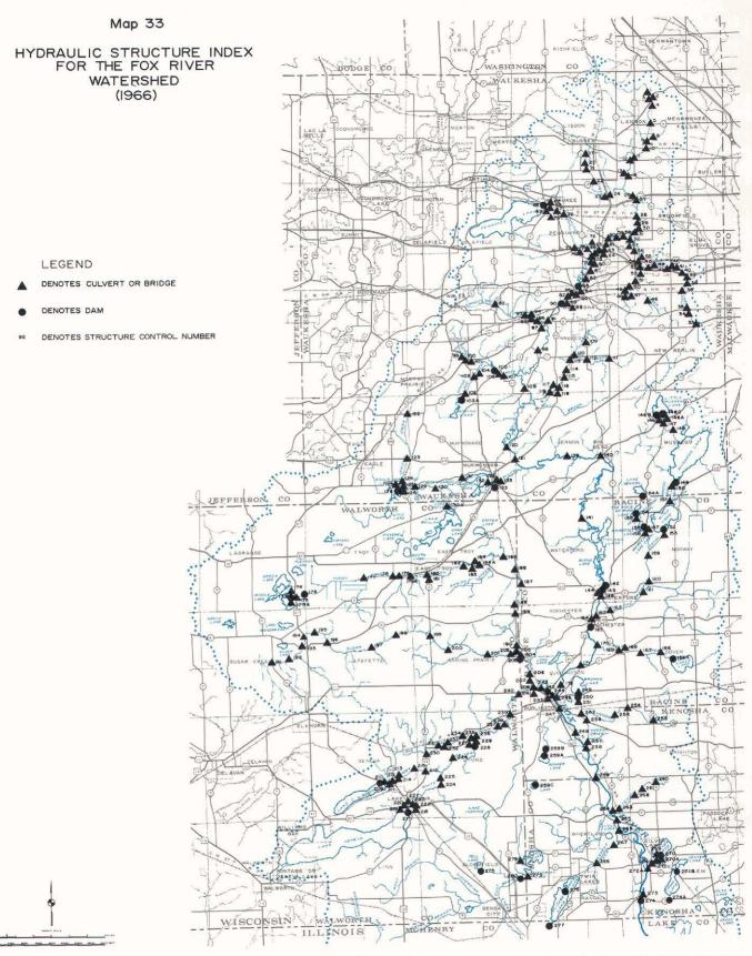
As a part of the hydraulic capacity inventory, the 251 bridges, culverts, and the 43 dams affecting the flow capacity of the Fox River drainage system were surveyed to establish the dimensions and capacity of each structure. In addition a second-order bench mark based upon mean sea level datum was established for each structure. *Source: SEWRPC*.
