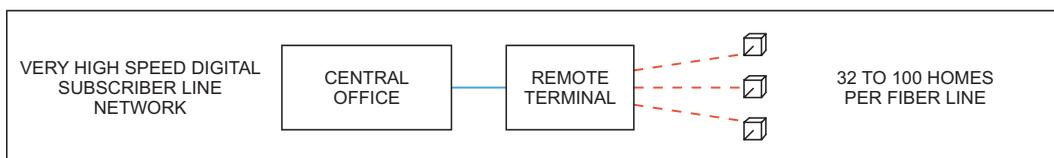
unchanged. The new element in DSL is a modem that converts data signals into a digital format for high speed transmission to the central office or remote terminal.
