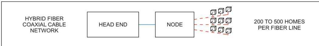
This joint sharing limits upload speeds to about 400 kilobits per second. As the number of users on each node rises, upload transmission rates are reduced. This asymmetric feature of broadband cable services, together with its inherent upper limit on transmission, makes hybrid fiber-coax a transition broadband communications technology.
