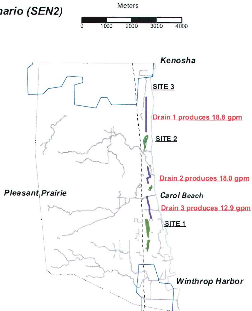
Figure 27. Scenario #3: Hypothetical drains for dewatering - location and simulated discharge.
