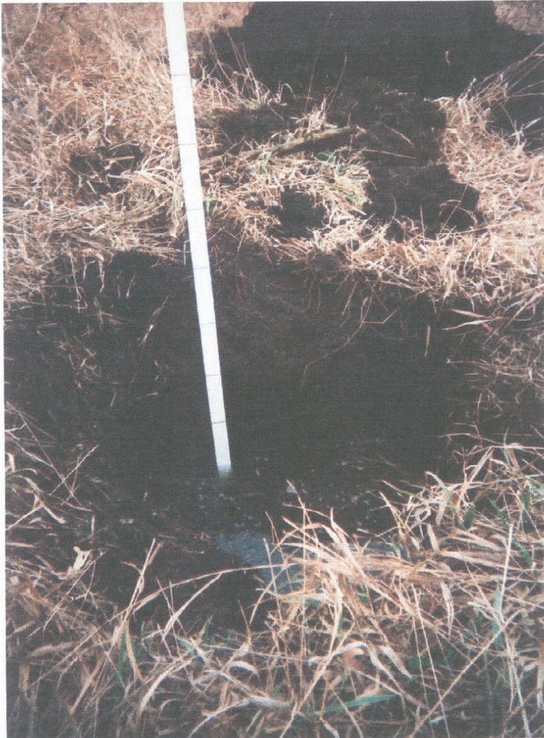
TEST PIT #4 – Concrete slab (3' x 2' x 4") on ground surface. No foreign material within soil profile. Groundwater encountered at 1 foot below grade. See Test Pit Log for soil profile description.
