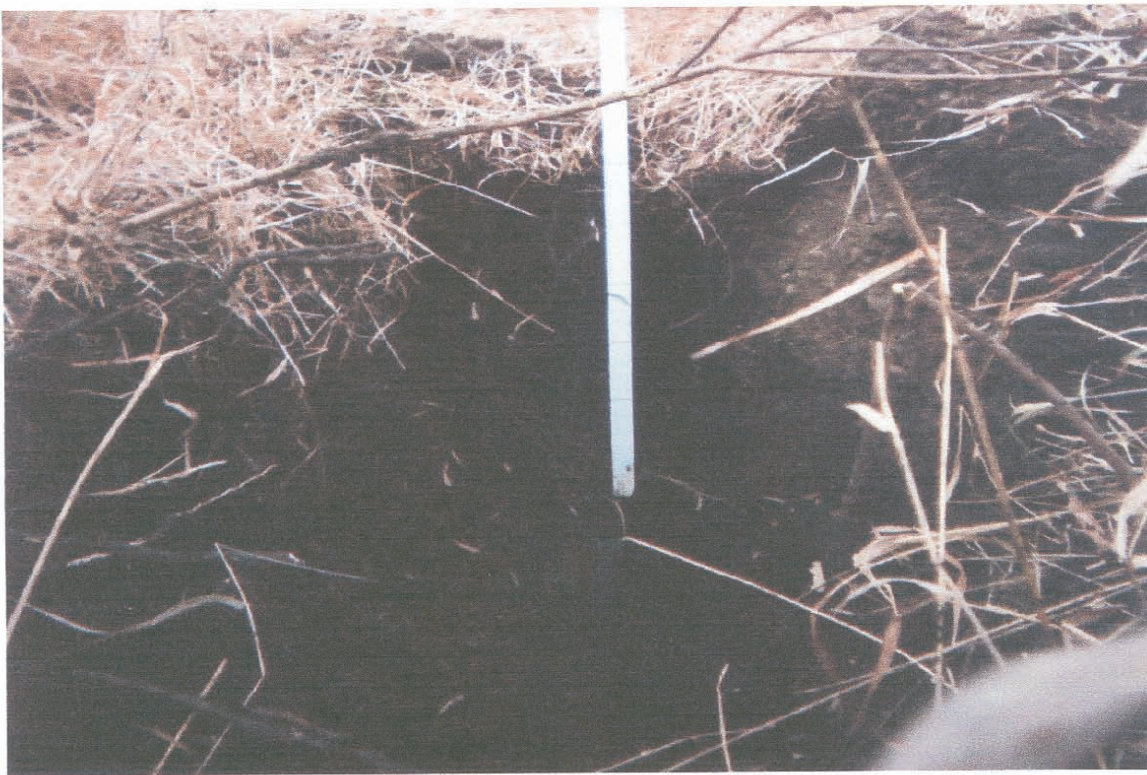
TEST PIT #2 – Concrete pieces on ground surface. No foreign material within soil profile. Groundwater encountered at 3 feet. See Test Pit Log for soil profile description.
