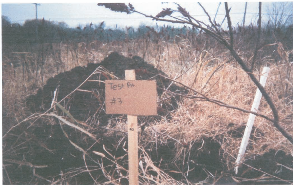
TEST PIT #3 – No foreign material within soil profile. Groundwater encountered at 2.5 feet below grade. See Test Pit Log for soil profile description.
