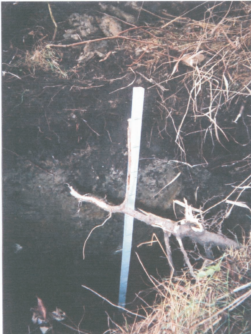
TEST PIT #8 – No foreign material within soil profile. Groundwater encountered at 2.5 feet below grade. See Test Pit Log for soil profile description.
