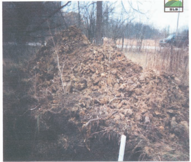
TEST PIT #7 – No foreign material in soil profile. Groundwater encountered at 3.5 feet below grade. See Test Pit Log for soil profile description.
