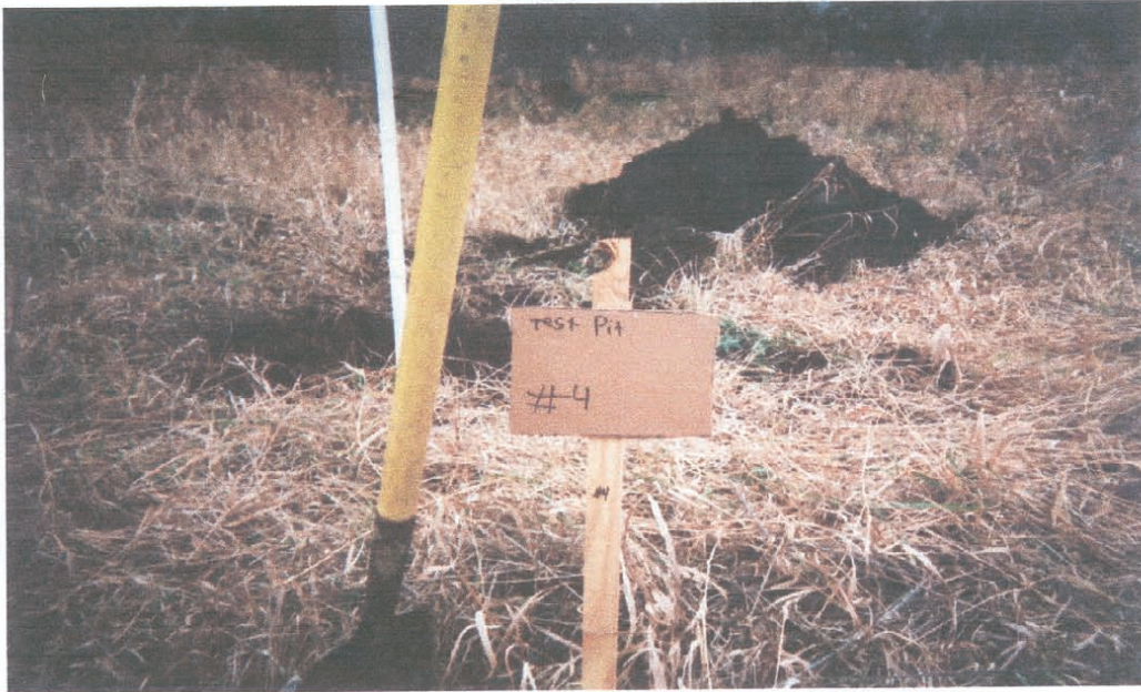
TEST PIT #4 – Concrete slab (3' x 2' x 4") on ground surface. No foreign material within soil profile. Groundwater encountered at 1 foot below grade. See Test Pit Log for soil profile description.
