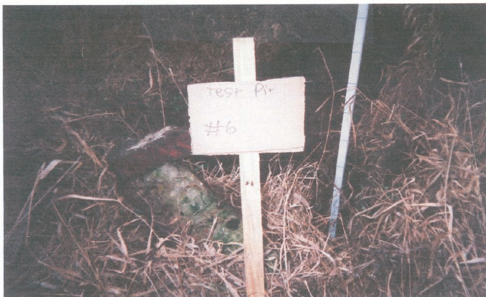
TEST PIT #6 – Small concrete pieces and red bricks on surface and within soil profile. Groundwater encountered 15” below grade. See Test Pit Log for soil profile description.
