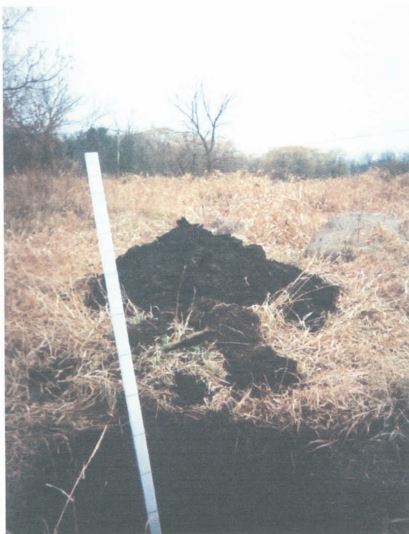
TEST PIT #3 – No foreign material within soil profile. Groundwater encountered at 2.5 feet below grade. See Test Pit Log for soil profile description.
