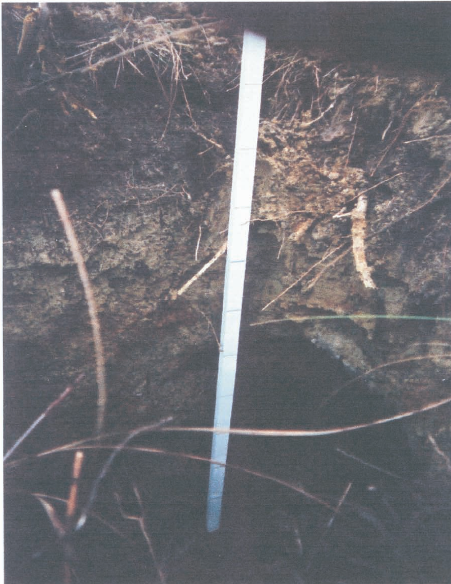
TEST PIT #7 – No foreign material in soil profile. Groundwater encountered at 3.5 feet below grade. See Test Pit Log for soil profile description.
