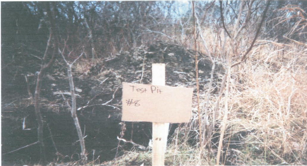
TEST PIT #8 – No foreign material within soil profile. Groundwater encountered at 2.5 feet below grade. See Test Pit Log for soil profile description.
