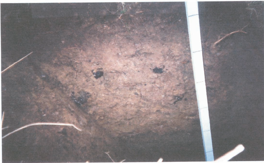
TEST PIT #1 – Note 4" to 6" asphalt pieces. Groundwater encountered at 3.5 feet below grade. See Test Pit Log for soil profile description.
