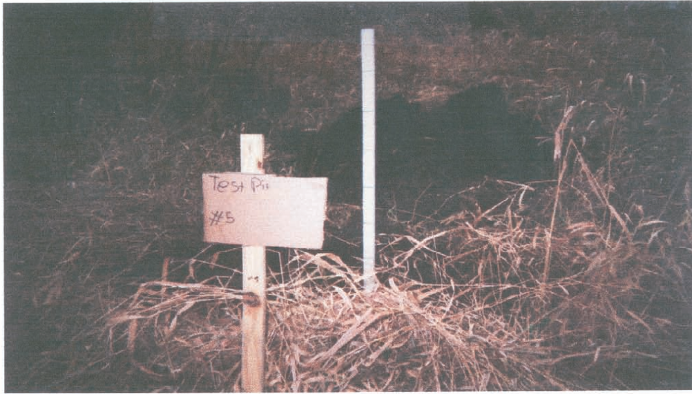
TEST PIT #5 – No foreign material within soil profile. Groundwater encountered at 2 feet below grade. See Test Pit Log for soil profile description.
