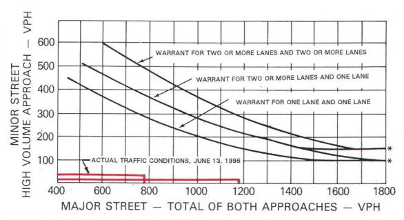
\*NOTE: 150 VPH APPLIES AS THE LOWER THRESHOLD VOLUME FOR A MINOR STREET APPROACH WITH TWO OR MORE LANES AND 100 VPH APPLIES AS THE LOWER THRESHOLD VOLUME FOR A MINOR STREET APPROACHING WITH ONE LANE.
