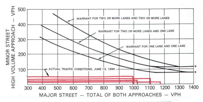
\*NOTE: 115 VPH APPLIES AS THE LOWER THRESHOLD VOLUME FOR A MINOR STREET APPROACH WITH TWO OR MORE LANES AND 80 VPH APPLIES AS THE LOWER THRESHOLD VOLUME FOR A MINOR STREET APPROACHING WITH ONE LANE.
