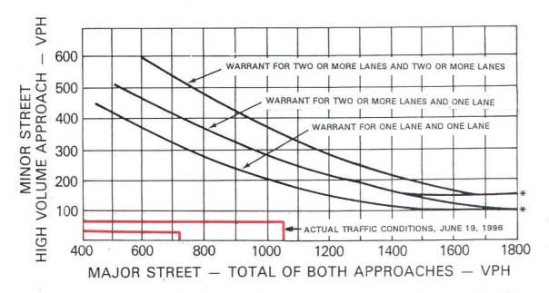
\*NOTE: 150 VPH APPLIES AS THE LOWER THRESHOLD VOLUME FOR A MINOR STREET APPROACH WITH TWO OR MORE LANES AND 100 VPH APPLIES AS THE LOWER THRESHOLD VOLUME FOR A MINOR STREET APPROACHING WITH ONE LANE.
