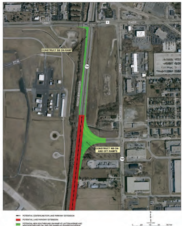
PREFERRED CROSSING TREATMENT FOR LAKE PARKWAY EXTENSION AT LAYTON AVENUE (CTH Y) AND EDGERTON AVENUE
