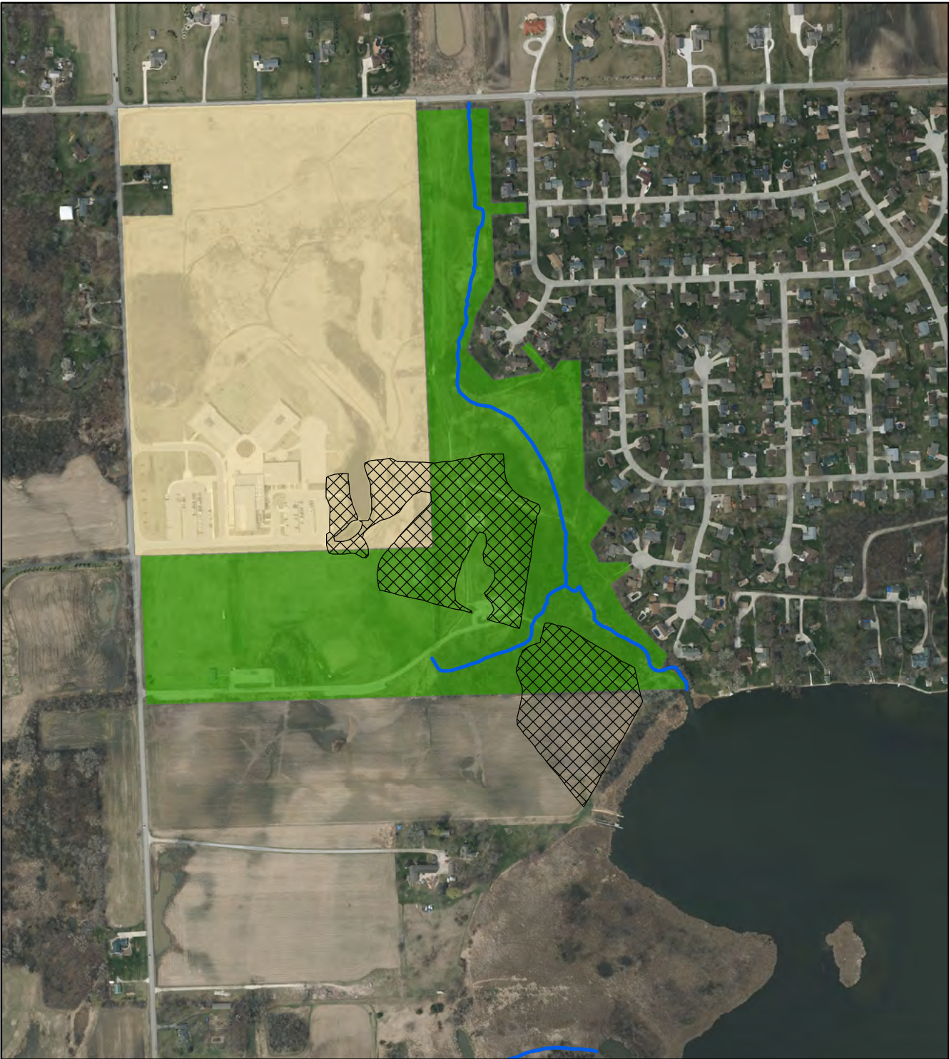
Map 3.1 Areas Underlain by Soils Favorable for Treatment Cell Construction and Operation: 2017
