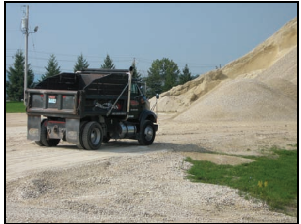
Having sources of aggregate relatively close (within 25 miles) of a construction project lessens the overall cost of construction due to the cost of transporting heavy materials.
