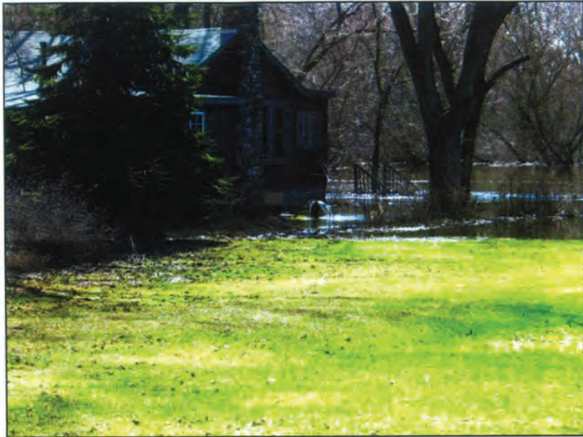
Flood waters surround one house and a vacant lot in the foreground. Owners of the house that once stood on the vacant lot opted to sell and move to drier land. The "fountain" of water next to the house is the well head. Hydrologic pressure is pushing the groundwater out the top.
