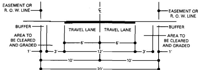
NOTE: CENTERLINES ARE NOT NORMALLY REQUIRED ON BICYCLE PATHS. WHERE CONDITIONS SUCH AS LIMITED SIGHT DISTANCE MAKE IT DESIRABLE TO SEPARATE TWO DIRECTIONS OF TRAVEL, A DOUBLE SOLID YELLOW LINE SHOULD BE USED TO INDICATE NO PASSING OR NO TRAVELING TO THE LEFT OF THE CENTERLINE.
