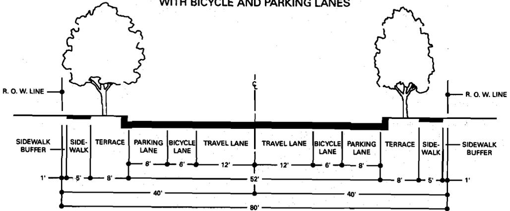
NOTE: A 6-INCH WIDE SOLID WHITE STRIPE SHOULD BE USED TO DISTINGUISH THE TRAVEL LANE FROM THE BICYCLE LANE. A 4-INCH WIDE SOLID WHITE STRIPE OR MARKED PARKING STALLS SHOULD BE USED TO DISTINGUISH THE BICYCLE LANE FROM THE PARKING LANE.
