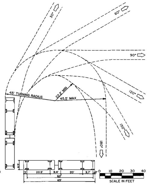
NOTE: The turning templates show the turning paths of the AASHTO design vehicles. The paths shown are for the left front overhang and the outside rear wheel. The left front wheel follows the circular curve, however, its path is not shown.
