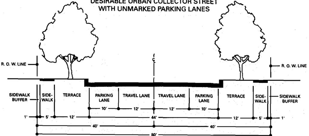
NOTE: IF THE RIGHT-OF-WAY WIDTH IS LIMITED, THEN THE TERRACE CAN BE REDUCED TO 7 FEET WIDE.
