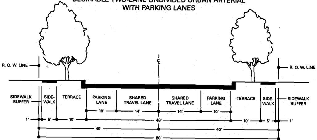
NOTE: A 4-INCH WIDE SOLID WHITE STRIPE OR MARKED PARKING STALLS SHOULD BE USED TO DISTINGUISH THE TRAVEL LANE FROM THE PARKING LANE.
