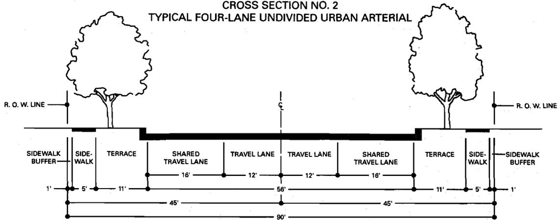
NOTE: IF THE RIGHT-OF-WAY WIDTH IS LIMITED, THEN THE TERRACE CAN BE REDUCED TO 6 FEET WIDE.
