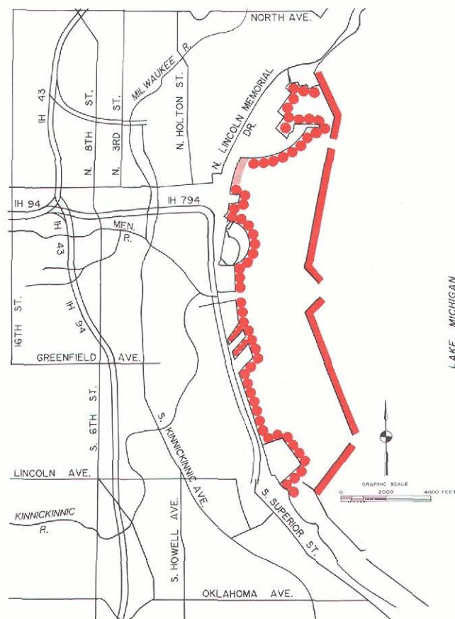
MILWAUKEE OUTER HARBOR BREAKWATER ALTERNATIVE NO. 2 RECONSTRUCT TO RAISE ELEVATION BY 8.7 FEET WITH POURED CONCRETE WALL
