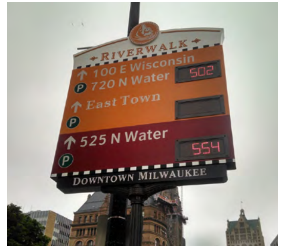
A Parking Guidance Sign Credit: City of Milwaukee
