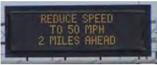
A Variable Message Sign Credit: WisDOT
