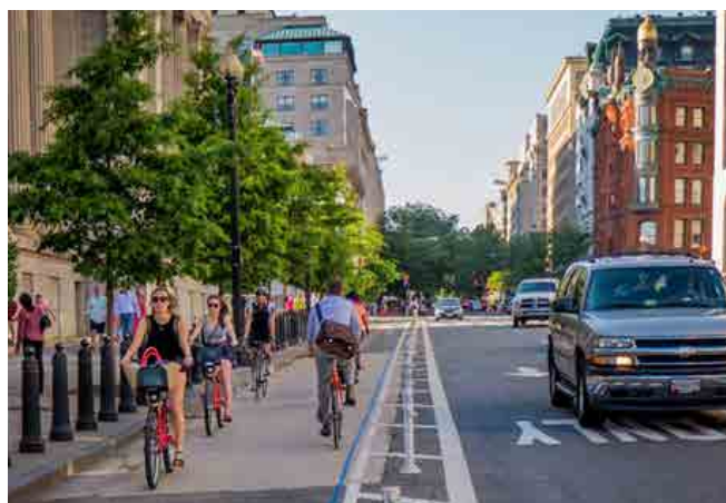
A two-way protected bike lane utilizing bollards in Washington, DC Credit: Stewart Eastep
