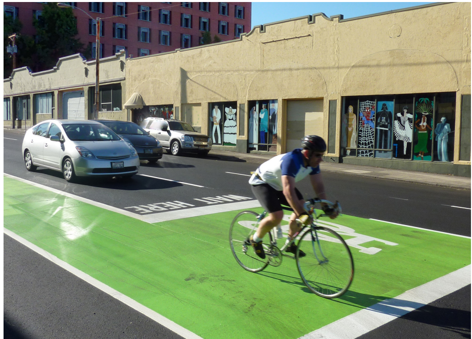
An intersection in Portland, OR utilizing a bike box at the head of a traffic lane Source: Otrec
