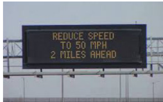
A Variable Message Sign Source: WisDOT
