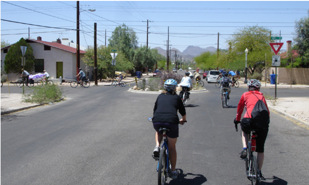
A neighborhood greenway utilizing a mini traffic circle to slow auto speeds on the corridor in Tucson, AZ. Source: NACTO
