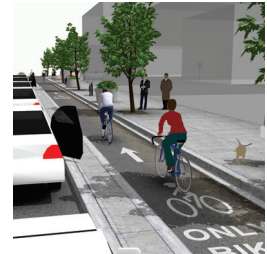
Protected Bike Lane
