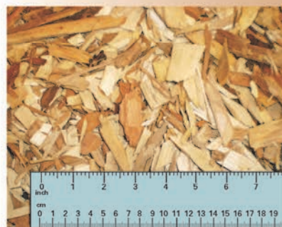
Figure 2. Woodchips commonly used in woodchip bioreactors
