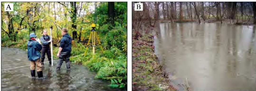
Figure 3. A: Measuring bankfull features in an urban stream. B: Bankfull flow in the same stream with water depths and currents that make taking measurements unsafe.
