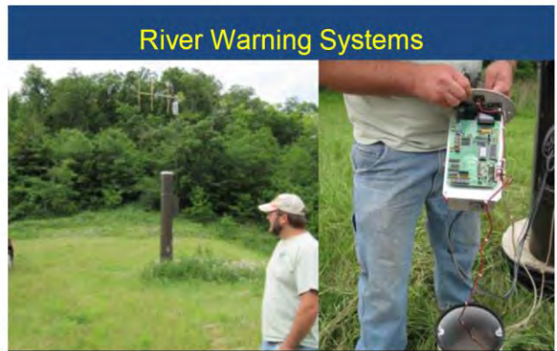
River warning systems installed on conservation dams to warn county officials about expected dam breaching. Images from Vernon County
